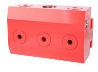
QH-2000TWS fluid ends are standardized products of our company for matching with the model 2000 power ends of fracturing truck produced by several fracturing equipment manufacturers in the world, and it has more than ten years' history in oilfield fracturing operation and it's durable in use.
